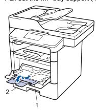
4. Slide the MP tray paper guides to fit the width of the paper you are using. If the paper guide on the right side has a lever, press it and slide the paper guide.
