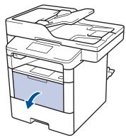
4. Pull out the MP tray support (1) and unfold the flap (2).
