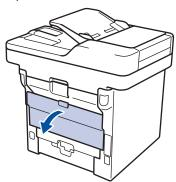
3. Pull the levers at the left and right sides toward you to release the fuser cover.
