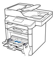
5. Load paper with the printing surface *face up* in the MP tray. When you use Letterhead or Preprinted paper, load the paper in the correct orientation as shown in the illustrations.
